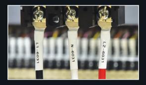
This non-adhesive tape is made of a special material that is wound in the tape cassette as a flat tube. Once printed on, the tube is opened up and passed over a cable or terminating connector. On heating with a heat gun, the tube shrinks to about half its original width, and in doing so grips the cable.
