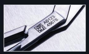
Brother stencil tape is used as part of an electro-chemical etching process to produce a mask containing the information to be etched. When an electrical current is passed through a pad containing specialist etching fluid, and pressed onto the stencil tape, it leaves a permanent mark with the text or barcode on the metal.
