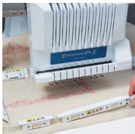
Included leverage magnet lifter, easy to remove the magnetic pieces
