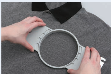
Set the garment in any direction, as long as the center of the frame is where you want it
