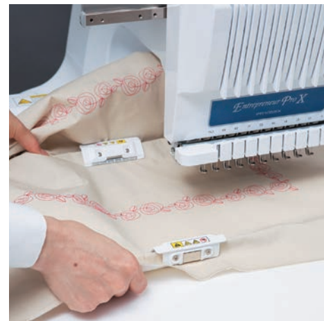
Easy to connect pattern, just slide the fabric on the frame to new area
