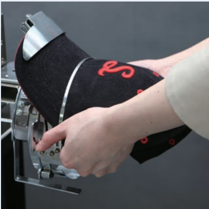
Stretch the cap over the frame
